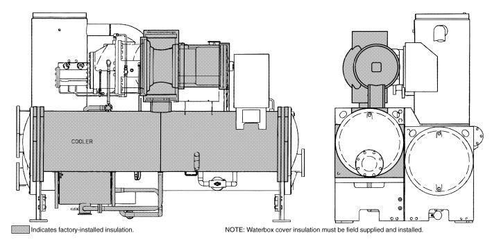
Fig. 32 — 23XL Insulation Area for Frame 1 and 2 Machines
